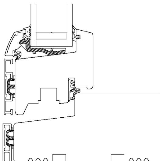
Figure 6. Type 2. Frame of wood plated with aluminium.
