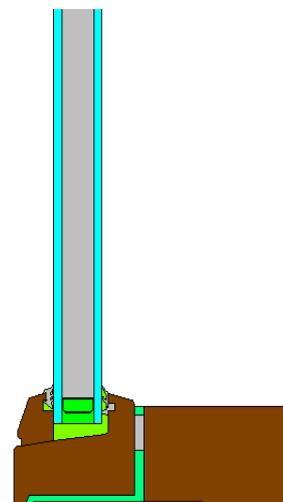
Figure 12. The wooden window with narrower sash, moved right down in front of the frame. A plastic sheet has been inserted in the frame to cover the thermal bridge insulation in the wall.
