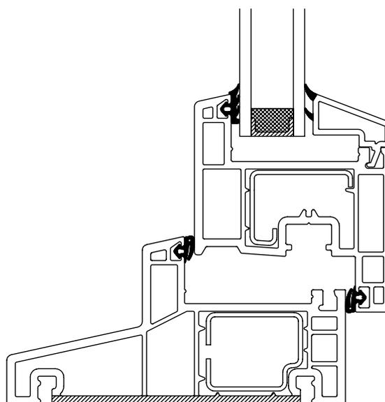
Figure 7. Type 3. Frame of plastic (left side facing outside).
