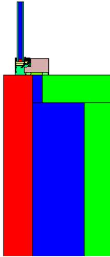
**Figure 13. Window med frame of mixed materials mounted in straight rebate (reference).**
