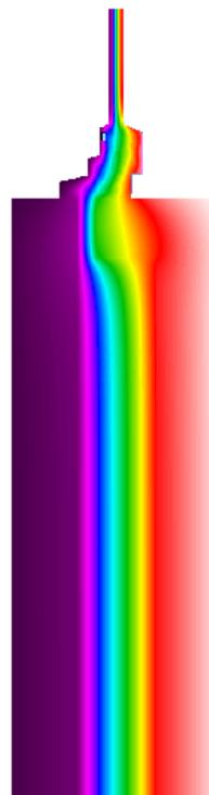
Figure 18. Isotherms in the construction. Frame of PVC.
