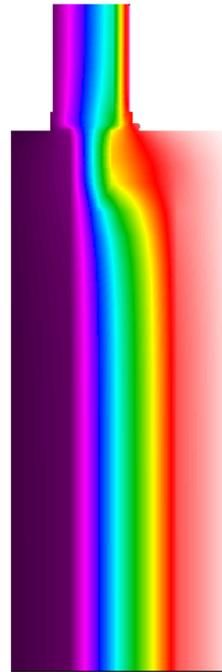
Figure 20. Isotherms in the construction with combination window.
