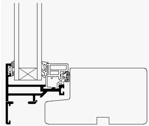
Figure 9. Type 5. Frame of mixed materials.
