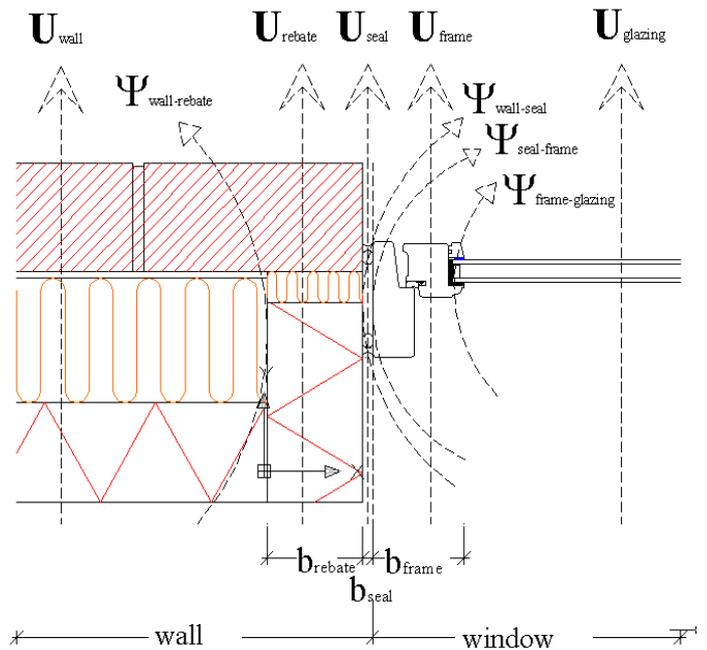
**Figure 3. Division of the expanded linear thermal transmittance between glazing and wall,  $L$ .**
