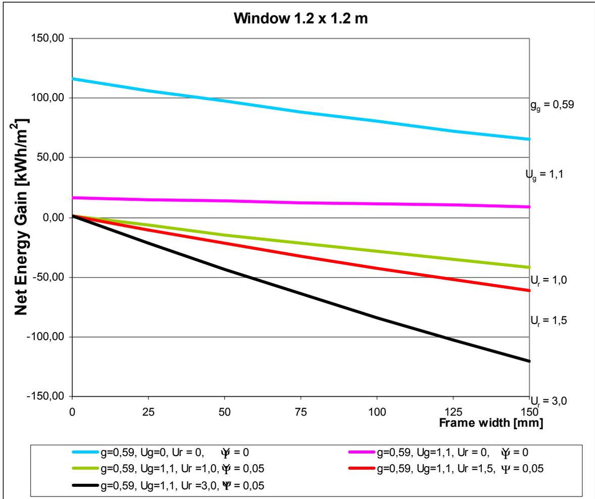
Figure 1. The net energy gain for different windows as a function of the frame width.
