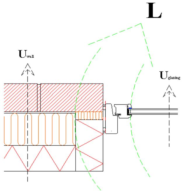
**Figure 2. The expanded linear thermal transmittance between glazing and wall**
