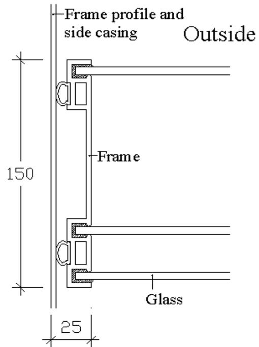
**Figure 10. Alternative frame construction made of fibre glass reinforced polyester and with space for 3 panes of glass.**
