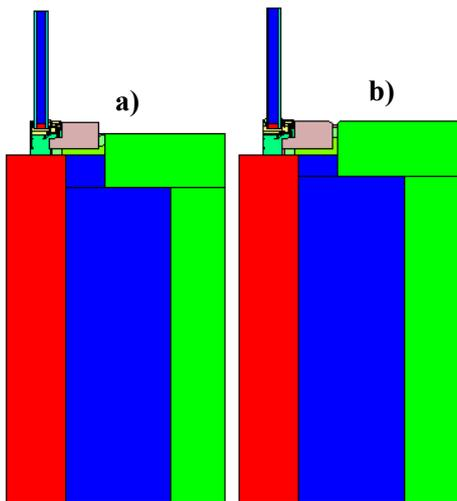
**Figure 14. Two examples of window with frame of mixed materials mounted in staggered rebate.**
