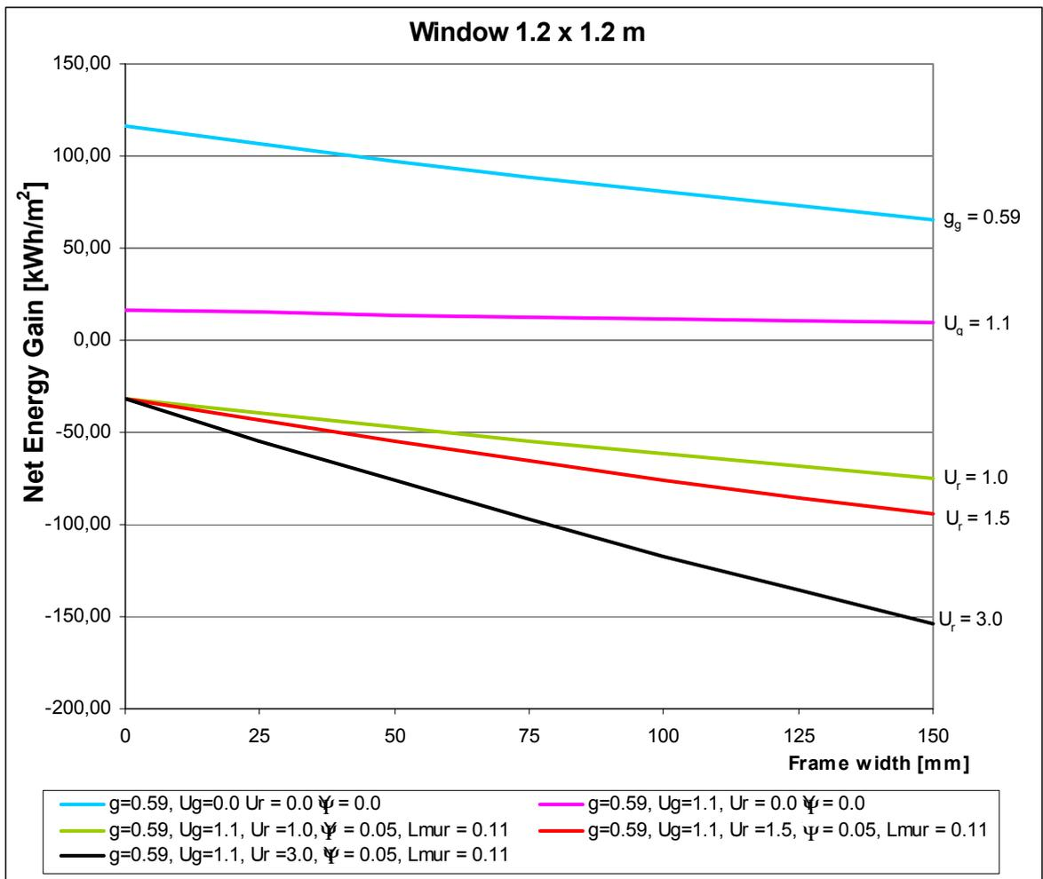
Figure 4. The net energy gain for different windows as a function of the width of the frame. The expanded linear thermal transmittance  $L_{mur}$  is included in the three lower curves.
