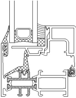
Figure 8. Type 4. Frame of aluminium.
