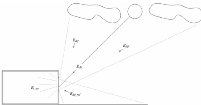
FIG. 1: The total light transmitted  $E_{t\_tot}$  is found with the visual transmittance and the illuminance on window from diffuse, reflected and direct sunlight.
