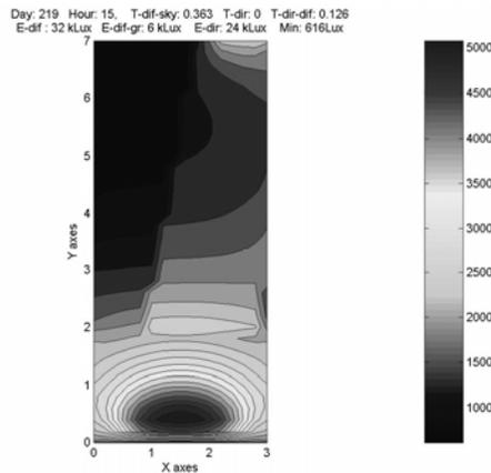
FIG. 4: Case with redirected sunlight reflected onto the ceiling. The reflected light increases the illuminance in the back of the room
