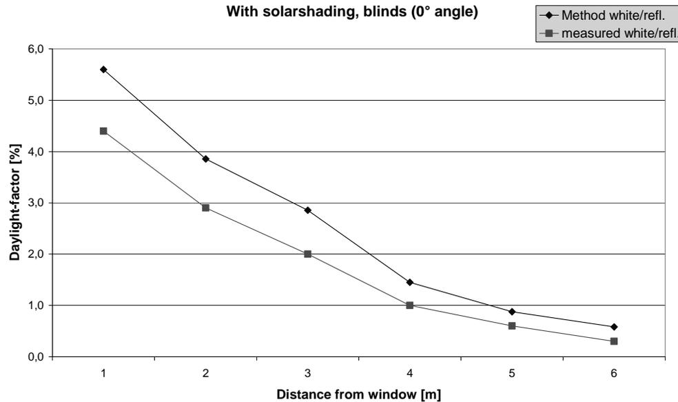
FIG. 6: Daylight-factors from method compared with daylight-factors from measurement. With solar shading device (blinds).
