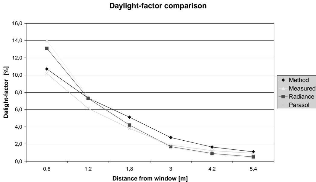
FIG. 5: Daylight-factors calculated by the presented method compared with measured daylight factors and daylight factors calculated with other simulation programs.
