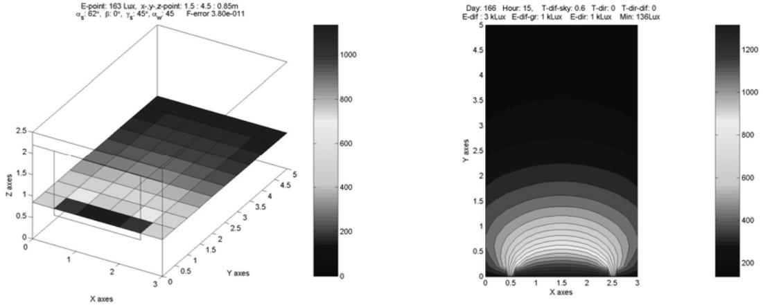
FIG. 3: Calculated results with developed method. The left window illustrates the position of the fictive horizontal plane showing the illuminance of each subsurface. The right window illustrates the same fictive plane with more accurate calculation.
