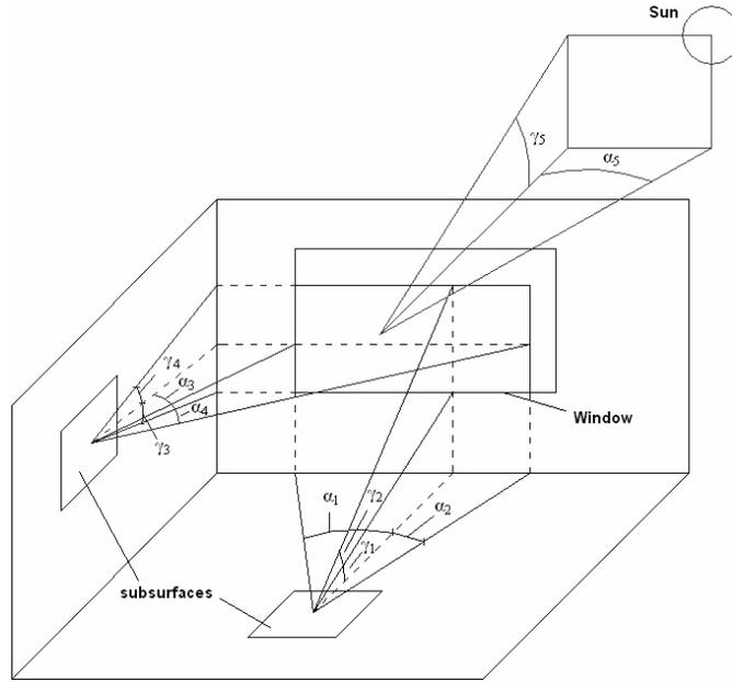
FIG. 2: A subsurface in a room is hit by direct sunlight if sun altitude ( $\gamma_s$ ) and azimuth ( $\alpha_s$ ) are within the view angles from the middle of the subsurface to window or shadow edges.
