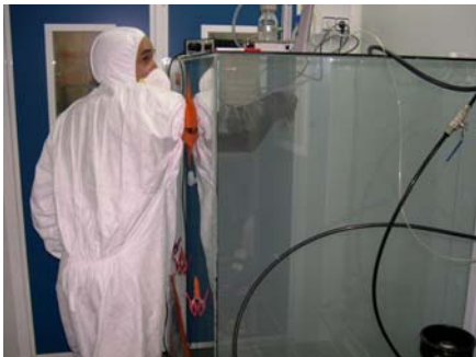
5 - Beads dispensing on closed room – before cholesteric liquid crystal filling.
