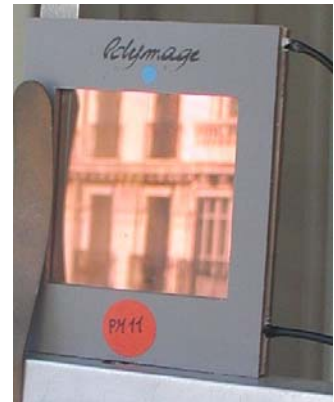
Figure 3d. Sample PM11: reflection view – return after U = 47V , f = 14 \text{ kHz} , for one minute.
