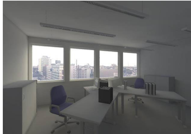
Figure 6. Office room with aerogel glazing. Illumination by a diffuse overcast sky.
