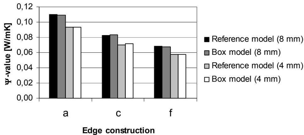
Figure 7: Variation of glass thickness from 4 mm to 8 mm in the wood frame profile with aluminium glazing bead.
