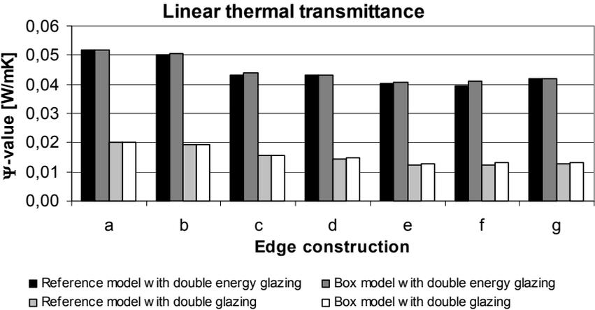
Figure 5: Linear thermal transmittance calculated for the reference model and the box model for an aluminium/wood/PVC frame profile with a double energy glazing and a double glazing.
