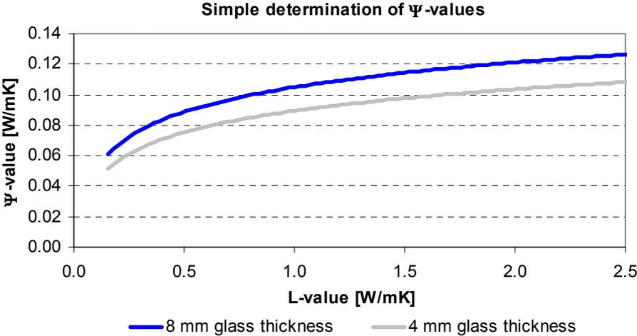
Figure 9: Diagram for simple determination of the linear thermal transmittance ( $\Psi$ -value). The diagram uses the thermal transmittance (L) of the edge construction and the glass thickness as input and is valid for a double energy glazing with a thermal transmittance applicable to the centre of the glazing ( $U_g$ ) of approximately  $1.2 \text{ W/m}^2\text{K}$ .
