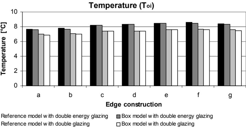
Figure 6: Temperature on the lower part of the inner glazing calculated for the reference model and the box model for an aluminium/wood/PVC frame profile with a double energy glazing and a double glazing.
