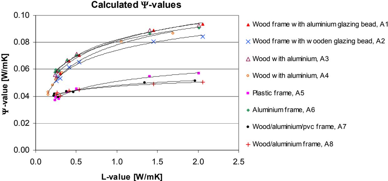
Figure 8: Calculated values of the linear thermal transmittance ( $\Psi$ -value). The diagram provides results for eight different frames as a function of the thermal transmittance (L) of the edge construction valid for a double energy glazing with a thermal transmittance applicable to the centre of the glazing ( $U_g$ ) of approximately  $1.2 \text{ W/m}^2\text{K}$ .
