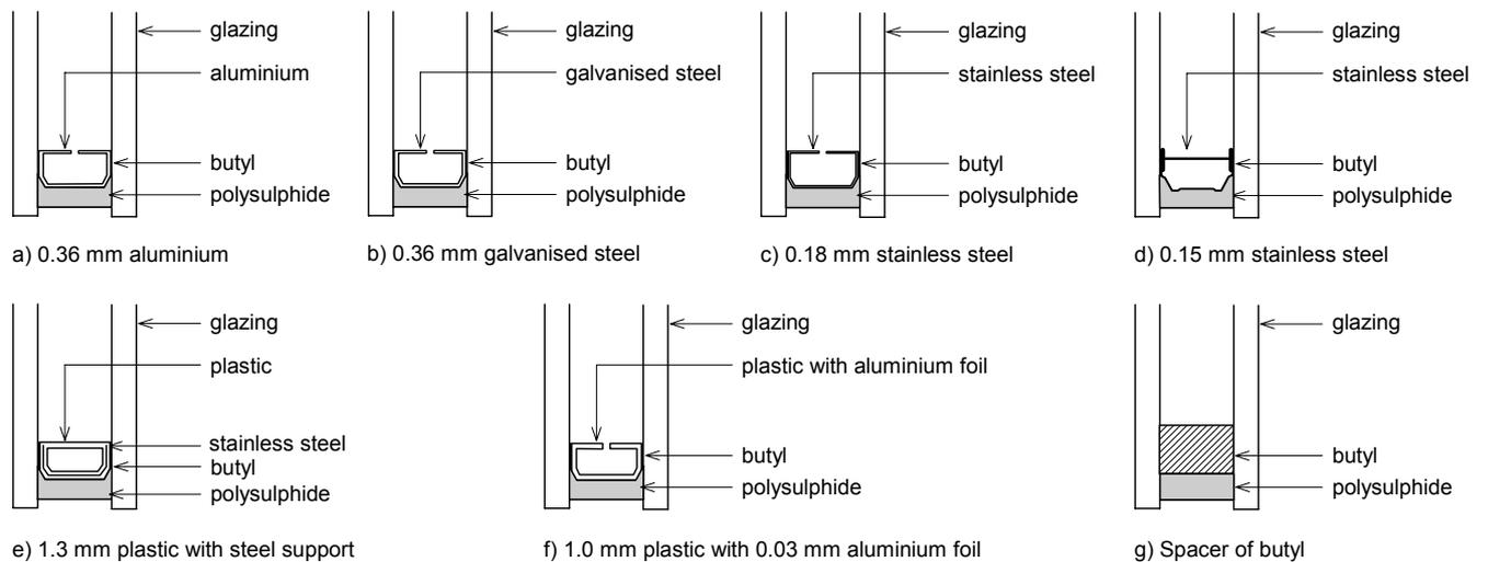
Figure 3: Sketch of the modelled edge constructions.
