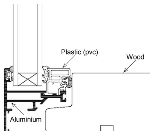
Figure 4: Sketch of the modelled frame profile made from aluminium, wood and PVC.
