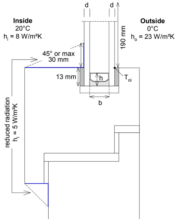
Figure 2: Sketch of the modified standard frame profile from (prEN ISO 10077-2) used to determine the equivalent thermal conductivity ( $\lambda_k$ ) in the box-model.
