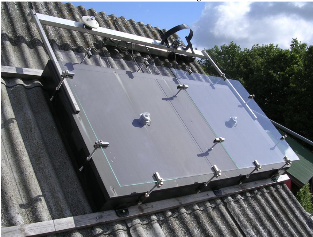
Fig. 4. Test facility used to measure the solar transmittance of two glasses. Left: Antireflection treated glass. Right: Normal glass.
