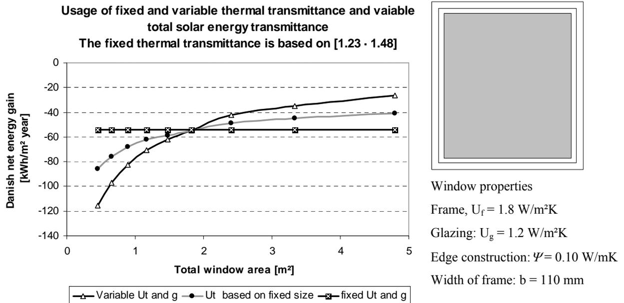
FIG. 1. Fixed or variable U- value combined with variable g-value
