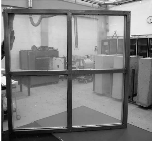
Fig. 6. Four optimized aerogel prototypes joined in a test frame for hotbox measurements.
